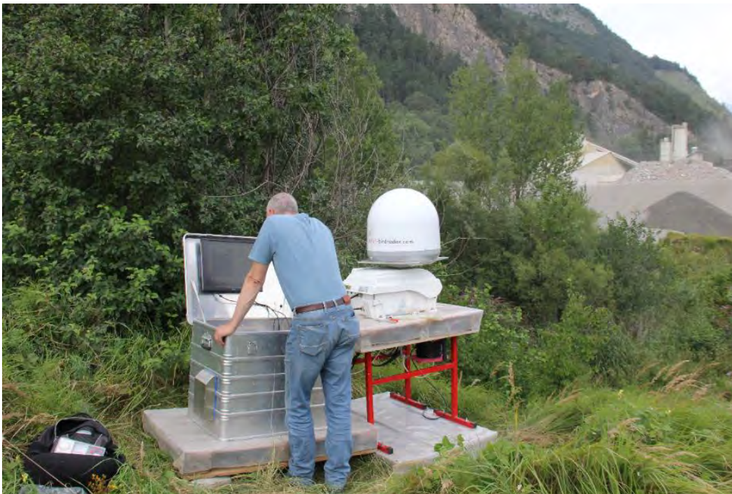
Fig. 10. Radar device model BirdScanMV1 on the rack at the right side with the radome (white dome) covering the antenna. The metal box contains the computer for the data registration and radar control.
